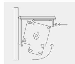
3. Once in the horizontal position tighten the bolt in each bracket, ensuring that the headrail is secure.
