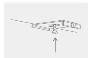
2. Attach the cassette to the bracket making sure it has caught the back lip of bracket as shown, and rotate into a horizontal position whilst keeping it tight against the bracket.
