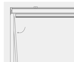
Press the adjustable sideguide into the fixed part, ensuring that the bottom bar will be free to move through it along the full drop of the blind.
