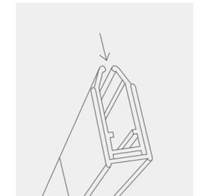
4. Slot bottom channel over the narrow part of the fixed sideguides as shown.
