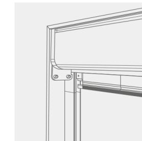
2. a) Press the top of the adjustable sideguide into the fixed part at an angle, as shown.
