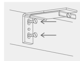
2. Attach the cassette to the bracket making sure it has caught the back lip of bracket as shown, and rotate into a horizontal position whilst keeping it tight against the bracket.
