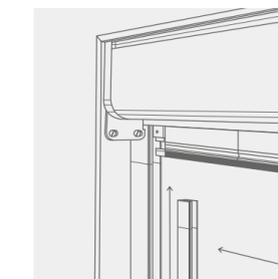
3. Press the adjustable sideguide into the fixed part, ensuring that the bottom bar will be free to move through it along the full drop of the blind.
