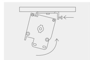
3. Once in the horizontal position tighten the bolt in each bracket, ensuring that the headrail is secure.
